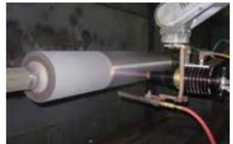
3. Flash carbide nano coating on piston rod
