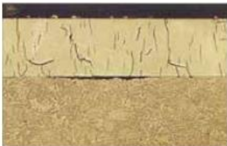
1. Hard chrome has micro cracks leading to pitting and corrosion
