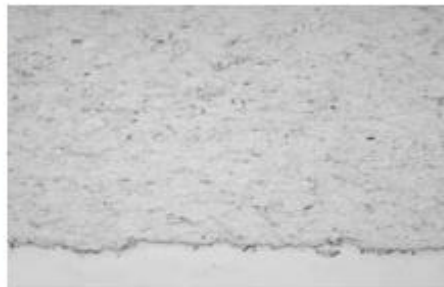
2. Flash carbide has no cracks and has less than 0.5% porosity and no through passage.
